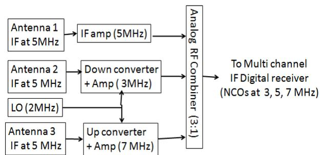
Fig 4: Three channel backend IF module.
