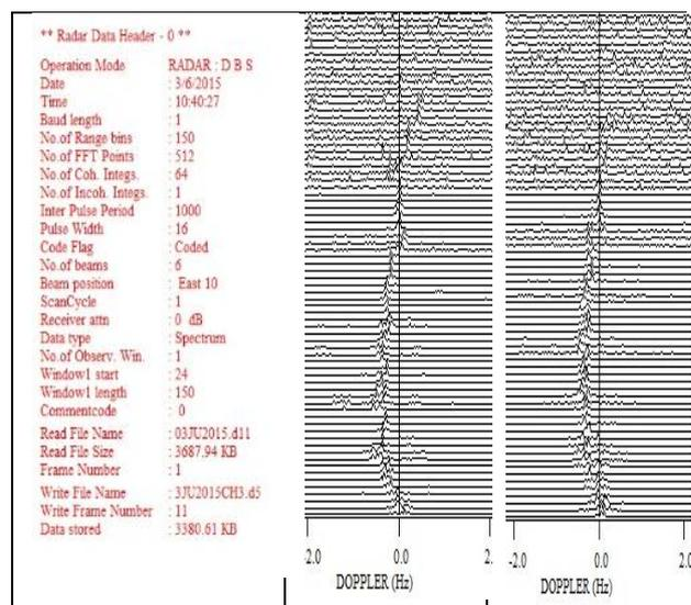
Fig 9: Comparison of 2d spectral plot of Single channel digital receiver and three-channel digital receiver, when both connected to MST Radar system parallel.
