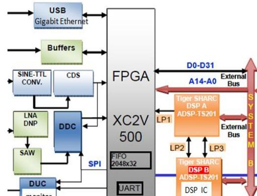
Fig: 2 Digital receiver block diagram
