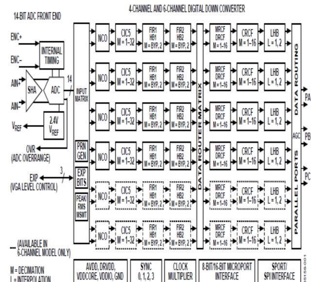
Fig3: AD6654 block diagram
