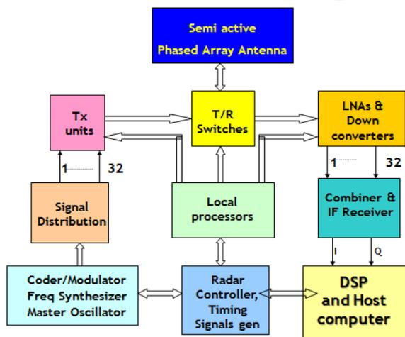
Fig1: MST Radar block diagram
